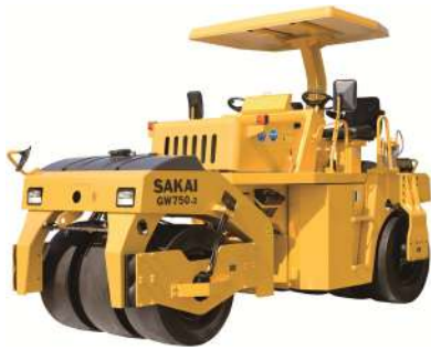
VIBRATORY PNEUMATIC TIRED ROLLER GW750-2 9,040Kg (19,930Lb)
