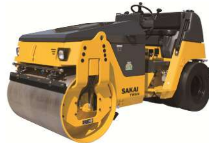
VIBRATORY DOUBLE DRUM ROLLER TW504 3,620Kg (7,980Lb)
