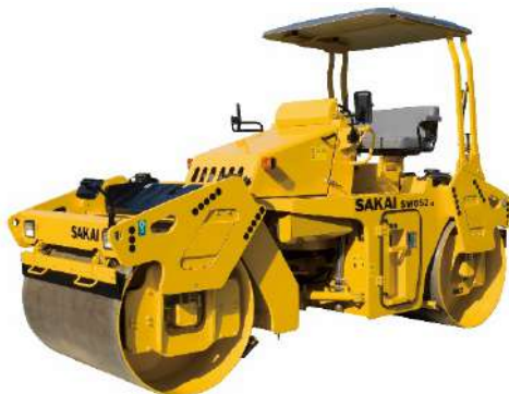
VIBRATORY DOUBLE DRUM ROLLER SW652/SW654 7,100Kg (15,650Lb)
