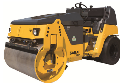
VIBRATORY DOUBLE DRUM ROLLER TW504 3,620Kg(7,980Lb)
