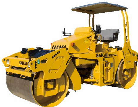
VIBRATORY DOUBLE DRUM ROLLER SW652/SW654 7,100Kg(15,650Lb)
