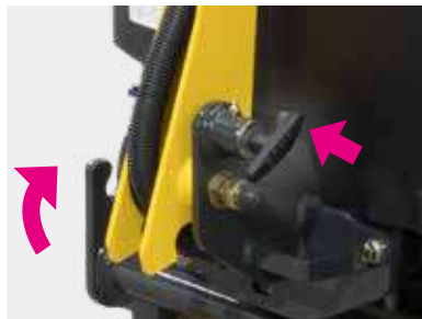
Locking pin for folding handle
