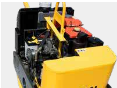
Full-open type cover for easy maintenance
