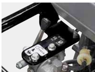
One throttle lever (Engine-off, Fuel-off, Throttle adjustment)
